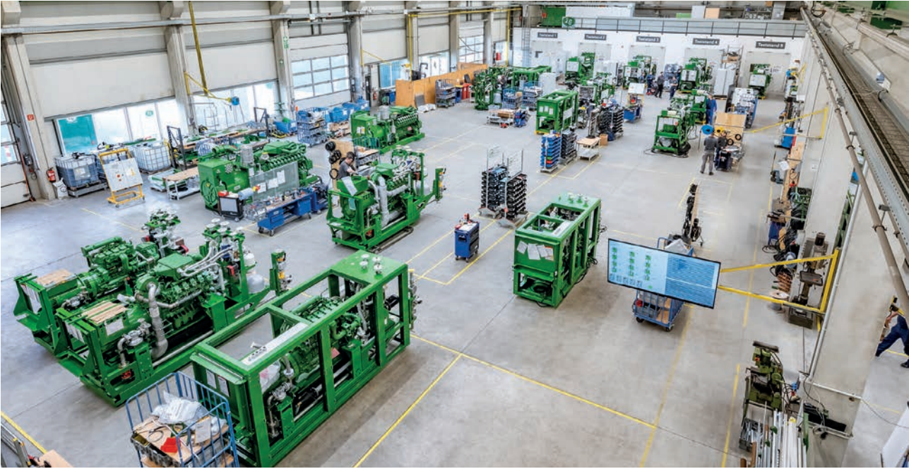
2G Energy manufactures CHP systems with electrical outputs ranging from 20 to 4,500 kW at its company headquarters in Heek/Germany
