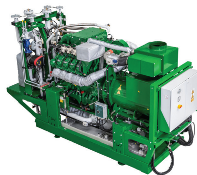
3. Enbridge Gas is building North America's first CHP system that will eventually run on 100% hydrogen to energize its Technology Operations Centre (TOC) in Markham, Ontario. The project's 115-kW 2G Agenitor engine will initially operate with a minimum blend of 25% hydrogen and 75% natural gas. Enbridge estimates the CHP system could consume approximately 78,000 kilograms of hydrogen annually. Courtesy: 2G
